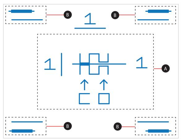
**Z-Gap** - The Z-Gap is the distance between the print pad and the print jet nozzles.
