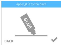
6. Apply two thin layers of Cube Glue to the print pad in an area of 50 mm x 50 mm. Select the **checkmark** to continue.
