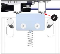
If the wiper blade is too high, remove the jet wiper assembly and turn the adjustment thumbscrew (A) clockwise. Reinstall the jet wiper and return to step 5.
