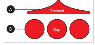
NOTE: Once all four corner Print Pad Level calibration points are correct, verify the Z-Gap to ensure that it is still correct.
