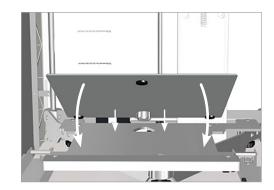
14. Mount the jet wiper mounting posts to the back panel of the printer through the keyhole slots.
