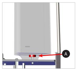
If the wiper tip is too low, remove the jet wiper assembly and turn the adjustment thumbscrew (A) counter-clockwise. Reinstall the jet wiper and return to step 5.
