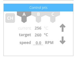
5. Once you have finished, reduce the target speed to 0.0 RPM and the target temperature to 0.0°C. You can now select the next print jet and follow this procedure if necessary.
