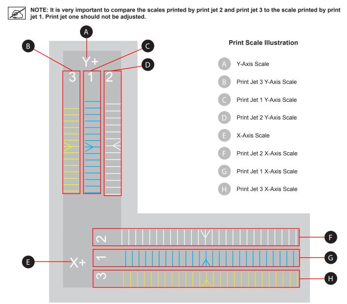
In the print scale illustration, the X+ scale (left-to-right) contains three (3) rows of printed lines. Each line represents a print jet. The prints are numbered 1, 2 and 3 for each of the three print jets. Print jet 1 always prints the middle scale so the scales of print jets 2 and 3 can be easily compared to it. Print jet 2 prints above print jet 1 and print jet 3 prints below print jet 1. For printers with only two (2) print jets, the scale below the print jet 1 scale will not be printed.
