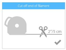
14. Cut off 2"/5 cm of print material from the end. Select the **checkmark** to continue.
